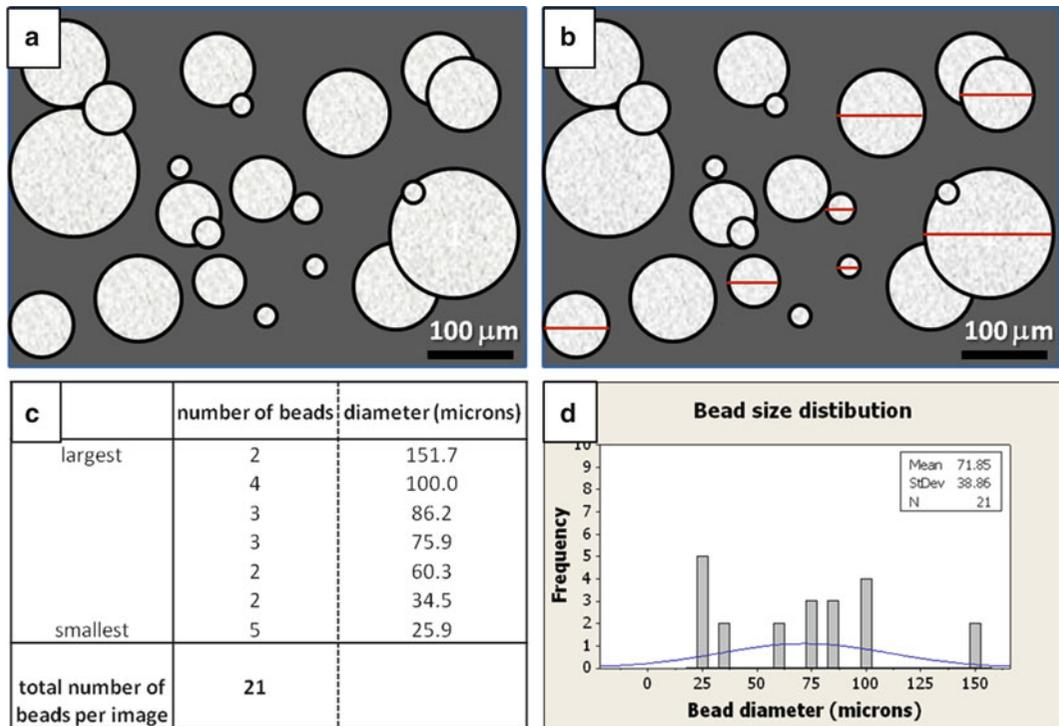
**Fig. 2** Methodology for bead size distribution determination. (a) Schematic of SEM image of beads; (b) illustration of bead diameter measuring procedure; (c) example of bead size and diameter compilation; (d) determination of bead size distribution
